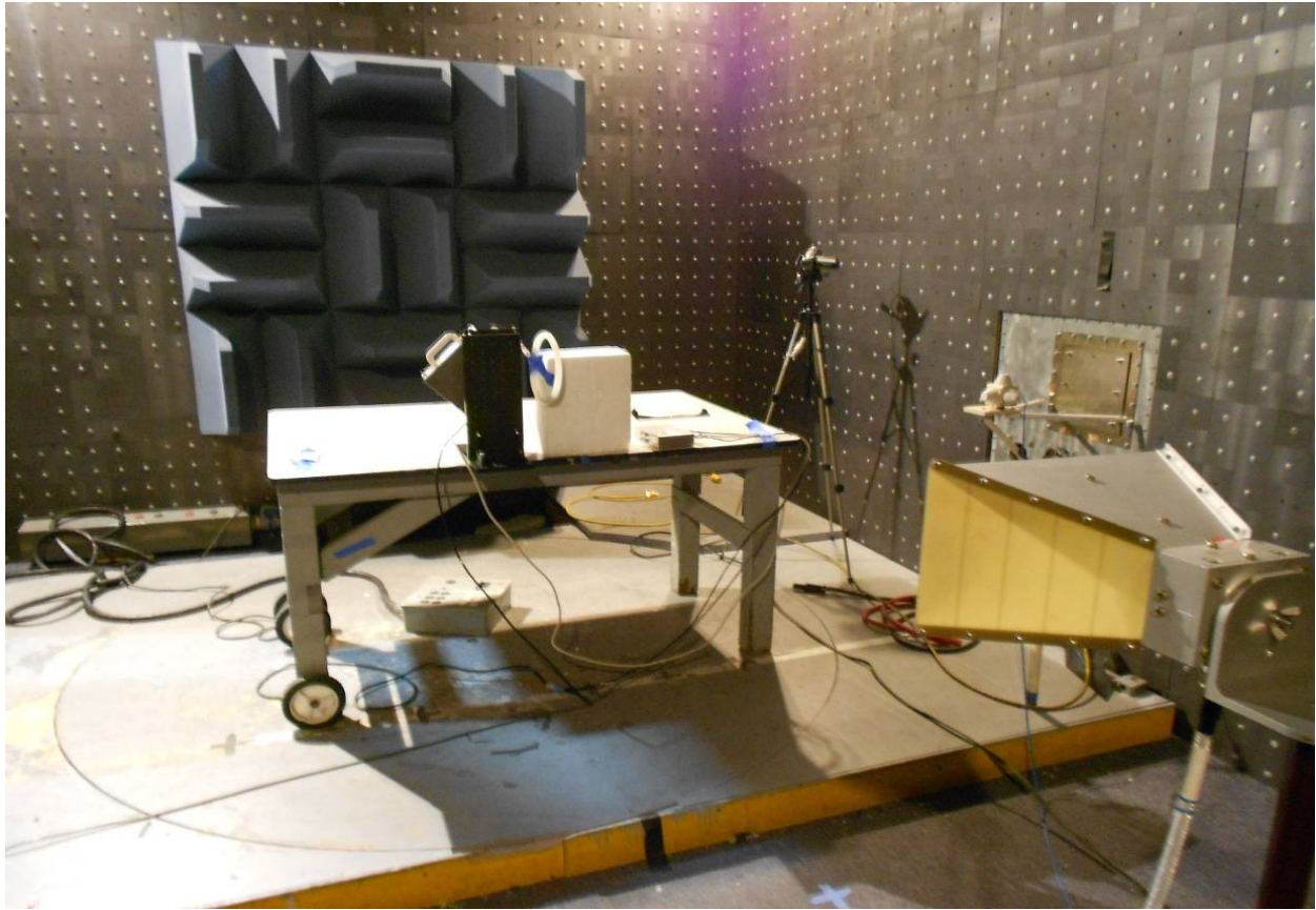
Test Configuration Photograph #2 (Radiated Immunity, EN 61000-4-3)
